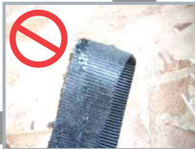
Figure 1: Unacceptable strap and attachment damage
